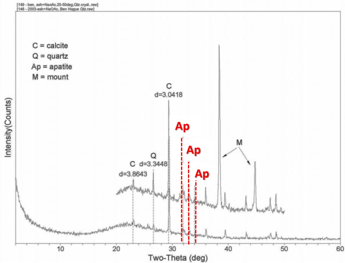
XRD analysis after salt and partial carbonate removal
